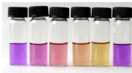
Figure 2. Color changes observed for the solution of 1 ( 5.0 \times 10^{-4} M) in the presence of different amounts of Gd 3+ and pyridine in CH 3 CN: from left to right: 0.0 equiv of Gd 3+ + 0.0 equiv of pyridine, 1.0 equiv of Gd 3+ + 0.0 equiv of pyridine, 2.0 equiv of Gd 3+ + 0.0 equiv of pyridine, 3.0 equiv of Gd 3+ + 0.0 equiv of pyridine, 4.0 equiv of Gd 3+ + 0.0 equiv of pyridine, 4.0 equiv of Gd 3+ + 4.0 equiv of pyridine.
